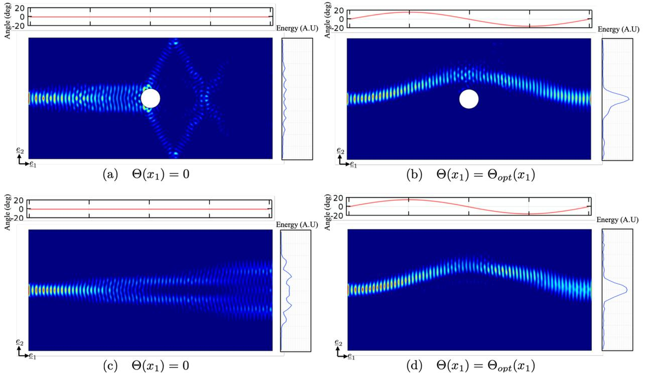
Figure 16: Four different case studies. On the left of each image the distribution of the energy at  $t = 700\mu s$ , on the right of each image the energy received at the right side of the specimen, in arbitrary units. Above each image the function  $\Theta_{opt}(x_1)$  is plotted.
