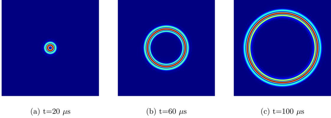
Figure 8: Snapshots of wave propagation for a high value of the exciting frequency (90 kHz) using a classic Cauchy model. Total displacement is displayed.
