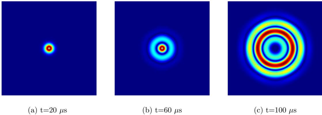
Figure 6: Snapshots of wave propagation for a low value of the exciting frequency (20 kHz) using a strain-gradient calibrated model. Total displacement is displayed.
