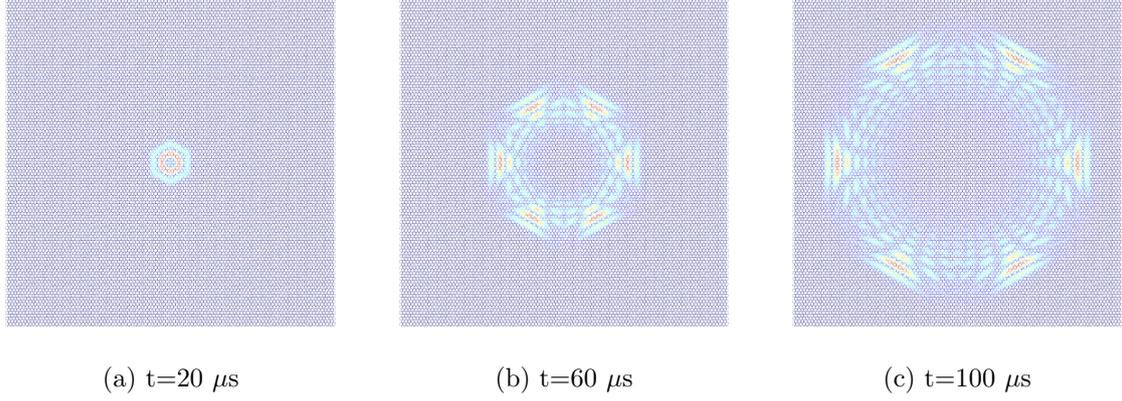
Figure 4: Snapshots a shear pulse at high frequency (90 kHz) for the honeycomb model ( $\eta \simeq 6$ ). The norm of the displacement is displayed, arbitrary units are used.
