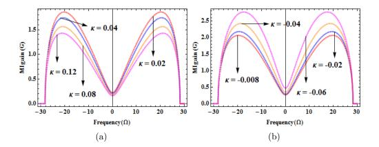
Figure 6: (Color online) The MI gain spectra for (a) different values of positive longitudinal diffraction  $\kappa$  and (b) for different values of negative longitudinal diffraction  $\kappa$  with other parameters as  $P_0 = 1$ ,  $\beta = 0.005$ ,  $\gamma_1 = 1$ ,  $\gamma_2 = 1$ , s = 0.004.
