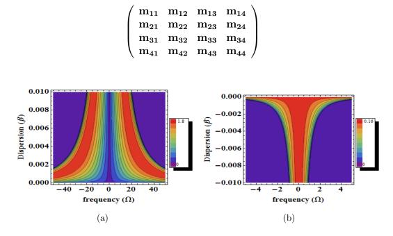
Figure 4: (Color online) The contour plots of MI spectra (a) in the anomalous dispersion regime, (b) the normal dispersion regime, with other parameters as  $\kappa = 0.005$  and s=0.002,  $P_0 = 1$ ,  $\gamma_1 = 1$ ,  $\gamma_2 = 1$ ,  $\mu = 2$ .
