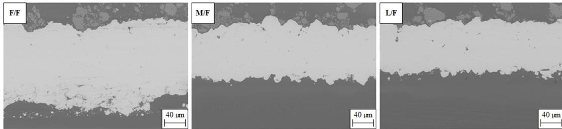
Figure 9: SEM cross section observations of F/F, M/F and L/F samples (800X)
