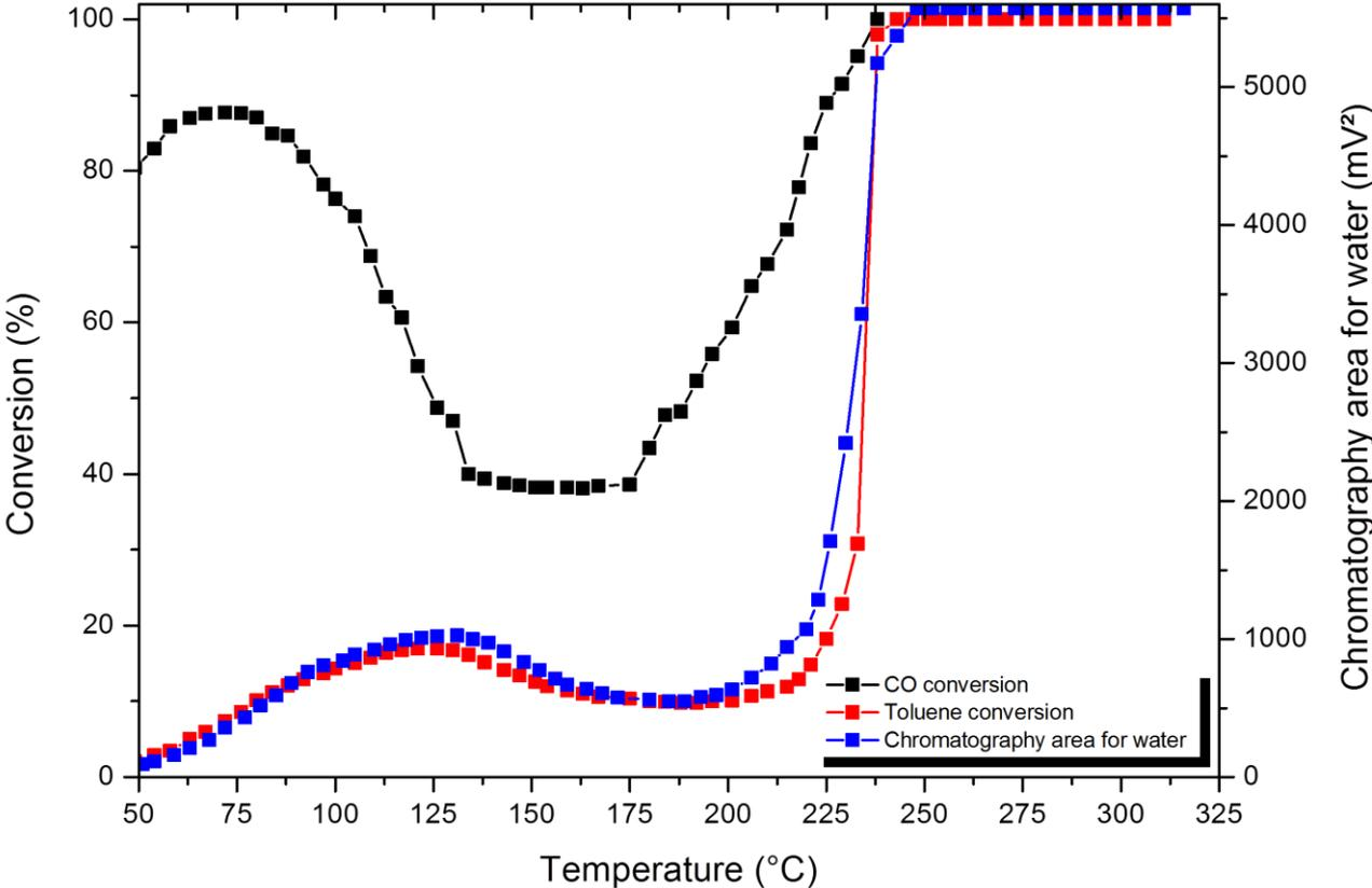
Figure 8 Influence of time on stream on the conversion of toluene on the CoAlOMW catalyst in presence of CO (Black) or in absence of CO (Red)
