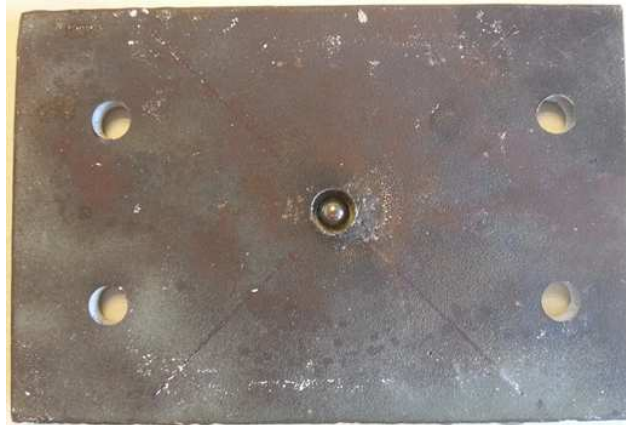
Figure 3. Specimen with the steel half ball placed for the test.
