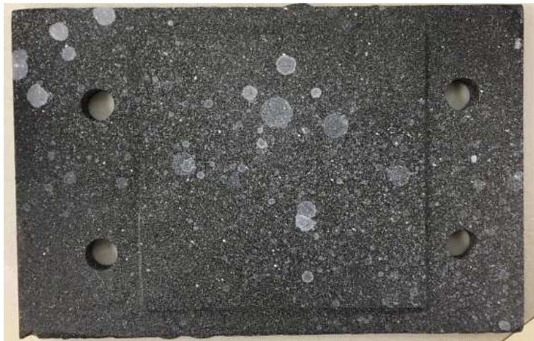
Figure 5. Specimen prepared for DIC.
