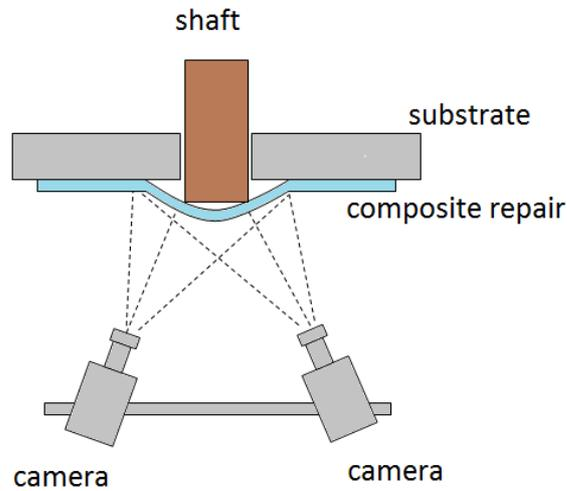
Figure 4. DIC schematic.
