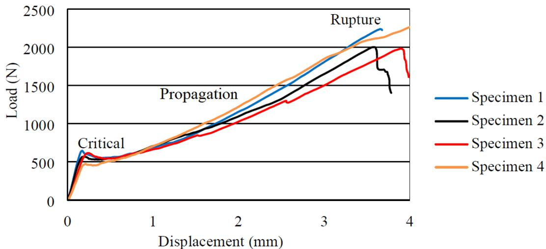
Figure 7. Blister tests - load displacement curves.
