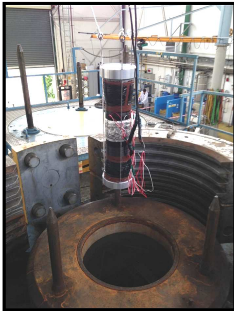
Figure 4 : 2400 bar pressure used for implosion test showing the 100 mm diameter C/PA6 cylinder just before test
