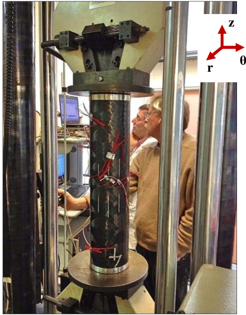
Figure 3: Axial compression test performed on a C/PA6 thermoplastic cylinder
