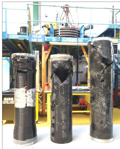
Figure 16: Composite cylinders after implosion tests - From left to right (i) C/PA6 [ \pm 0/88 ] (ii) C/PA6 [ \pm 55 ] (iii) C/Epoxy [ \pm 55 ]
