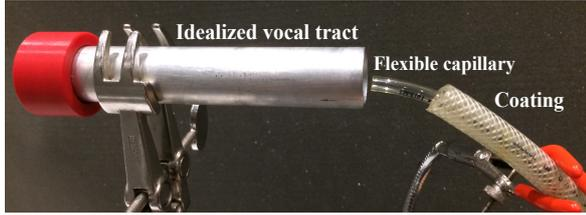
Figure 1 – Photo of excitation at the waveguide inlet.
