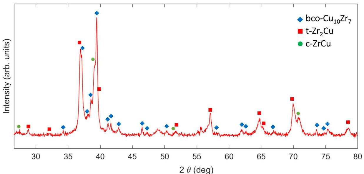
FIG. 6: Post-mortem XRD diffractogram of partially crystallized  $\text{ZrCu}$  thin films, showing evidence of body-centered orthorhombic  $\text{Cu}_{10}\text{Zr}_7$ , tetragonal  $\text{Zr}_2\text{Cu}$ , and cubic  $\text{ZrCu}$  phases. The crystallization fraction is observed to be approximately 80%.
