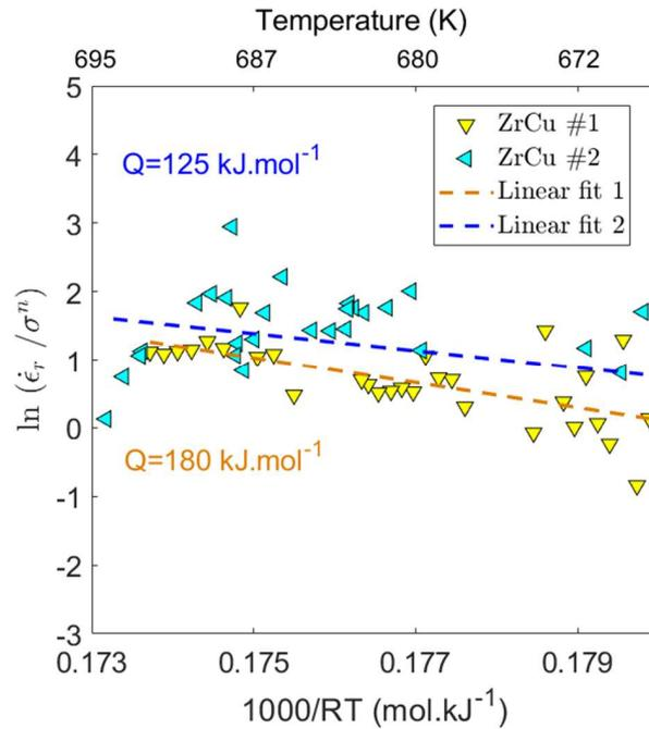
FIG. 5: Determination of the activation energy for creep deformation for the supercooled liquid region of ZrCu TFMGs from the linear fitting of  $\ln(\dot{\epsilon}_r/\sigma^n)$  versus  $1/RT$ .
