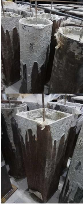
(b) CFST columns after casting
