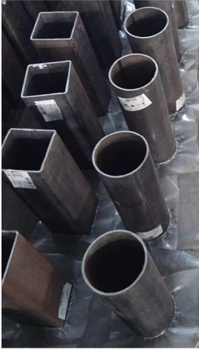
(a) Steel tubes prepared for casting
