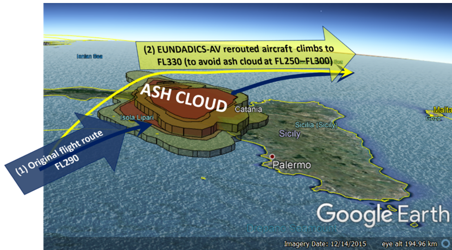
Figure 15. Example of a rerouting of one flight calculated by FLIGHTKEYS and simulated with NAVSIM/USBGSim (University of Salzburg), laterally and vertically avoiding volcanic ash (red \geq 4 \text{ mg m}^{-3} , yellow 2\text{--}4 \text{ mg m}^{-3} , green 0.2\text{--}2 \text{ mg m}^{-3} at different flight levels), © Google Earth.
