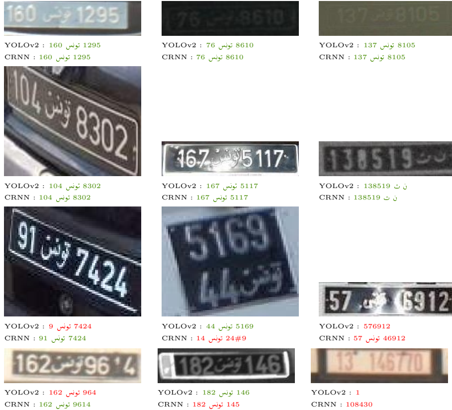
Figure 9: Qualitative results obtained by the proposed ALPR system in the GAP-LP and Radar datasets. Green text refers to correctly recognized LP, while miss-recognized LP are written in red.
