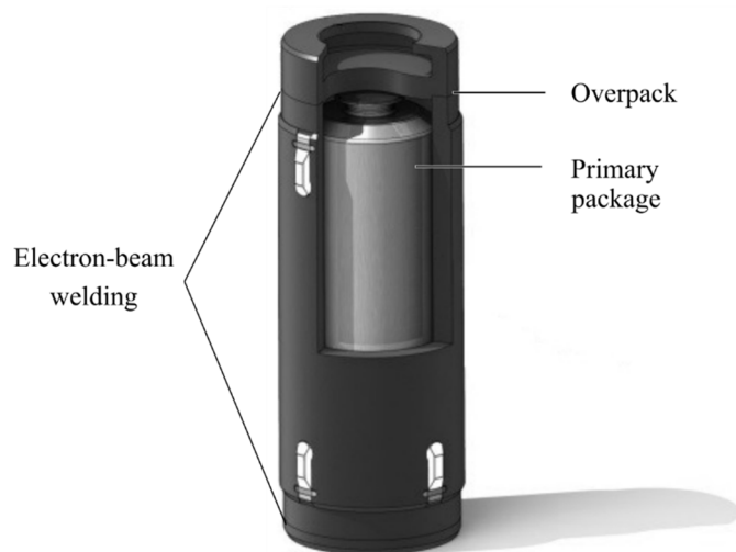
Figure 2. R7-T7 vitrified waste disposal package
