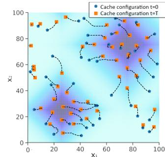
Fig. 1: Cached objects’ movements in the representation space ( $\mathbb{R}^2$ ) during  $[0, T]$  when the cache is managed by GRADES. The catalog is made by the points in a  $100 \times 100$  grid, dark shaded areas correspond to more popular objects. Dissimilarity cost  $C_d(x, y) = 1/10\|x - y\|_1$ , retrieval cost  $C_r = 1$ , cache size  $k = 50$ . See the description in Sect. V.
