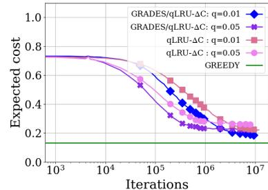
Fig. 8: Expected cost  $\mathcal{C}(\cdot)$  incurred by the different caching policies for the trace *360° videos* in Table I. GRADES/ $qLRU-\Delta C$  ( $q = 0.01, 0.05$ ) with  $\eta = 1.0$  and  $qLRU-\Delta C$  ( $q = 0.01, 0.05$ ). Cache size  $k = 4000$ .
