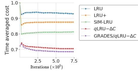
Fig. 9: The time averaged cost incurred by different policies under the trace *Amazon trace*: LRU, LRU+, SIM-LRU,  $q\text{LRU}-\Delta C$  ( $q = 10^{-3}$ ) and  $\text{GRADES}/q\text{LRU}-\Delta C$  ( $\eta = 6.9 \times 10^2$ , grafted with  $p = 1$ ). The level of approximability is 10%. Cache size  $k = 100$ .
