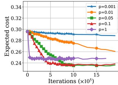
Fig. 6: Effect of grafting parameter  $p$  on the expected cost  $\mathcal{C}(\cdot)$  in a dynamic setting for GRADES/ $qLRU-\Delta C$  ( $\eta = 0.64$ ). The cache is initialized to a stationary configuration as in Fig. 3. Now, only requests corresponding to region B from the synthetic trace are made. Cache size  $k = 313$ .
