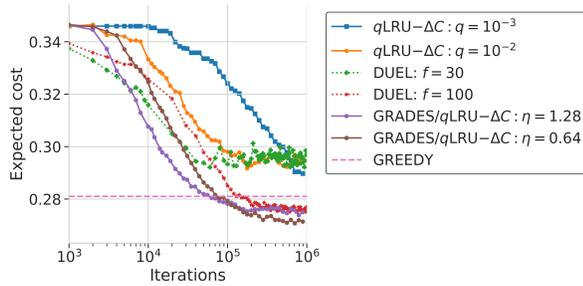
Fig. 7: Expected cost  $\mathcal{C}(\cdot)$  incurred by the different policies under the trace *Synthetic* in table I:  $qLRU-\Delta C$  ( $q = 10^{-3}, 10^{-2}$ ), DUEL, GREEDY, and GRADES ( $\eta = 1.28, 0.64$ ) grafted with  $p = 1$  and  $q = 10^{-3}$ . Cache size  $k = 313$ .
