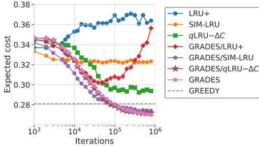
Fig. 4: Expected cost  $\mathcal{C}(\cdot)$  incurred by different policies under the trace *Synthetic* in Table I: LRU+, SIM-LRU,  $qLRU-\Delta C$  ( $q = 10^{-2}$ ), GREEDY, and GRADES ( $\eta = 0.64$ , plain and grafted with  $p = 10^{-1}$ ). Cache size  $k = 313$ .
