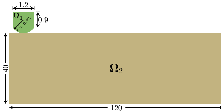
Figure 9: The geometry of the shallow ironing problem
