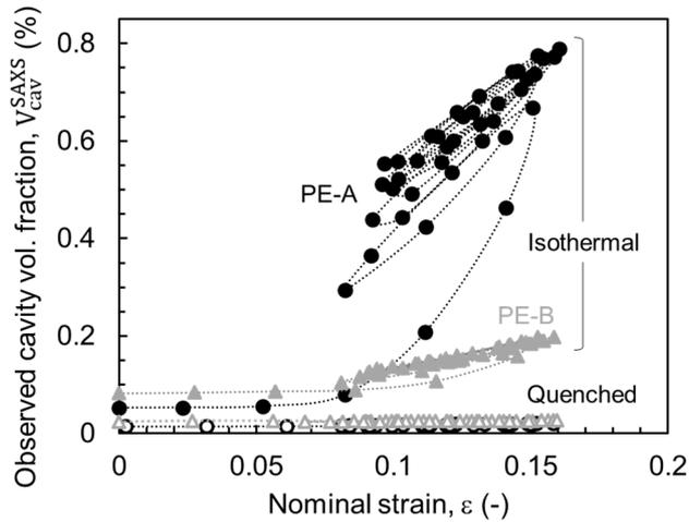
**Figure 7:** Evolution of the observed cavity volume fraction  $V_{cav}^{SAXS}$  as a function of the imposed nominal axial strain during oligo-cyclic test.
