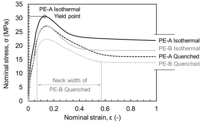
**Figure 1** : Tensile curves and measurement of neck width
