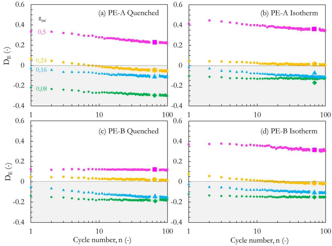
**Figure 9:** Relative change of the secant modulus evaluated by  $D_E$  as a function of cycle number in PE samples with different applied oligo-cyclic strains: (a) PE-A Quenched; (b) PE-A Isothermal; (c) PE-B Quenched and (d) PE-B Isothermal
