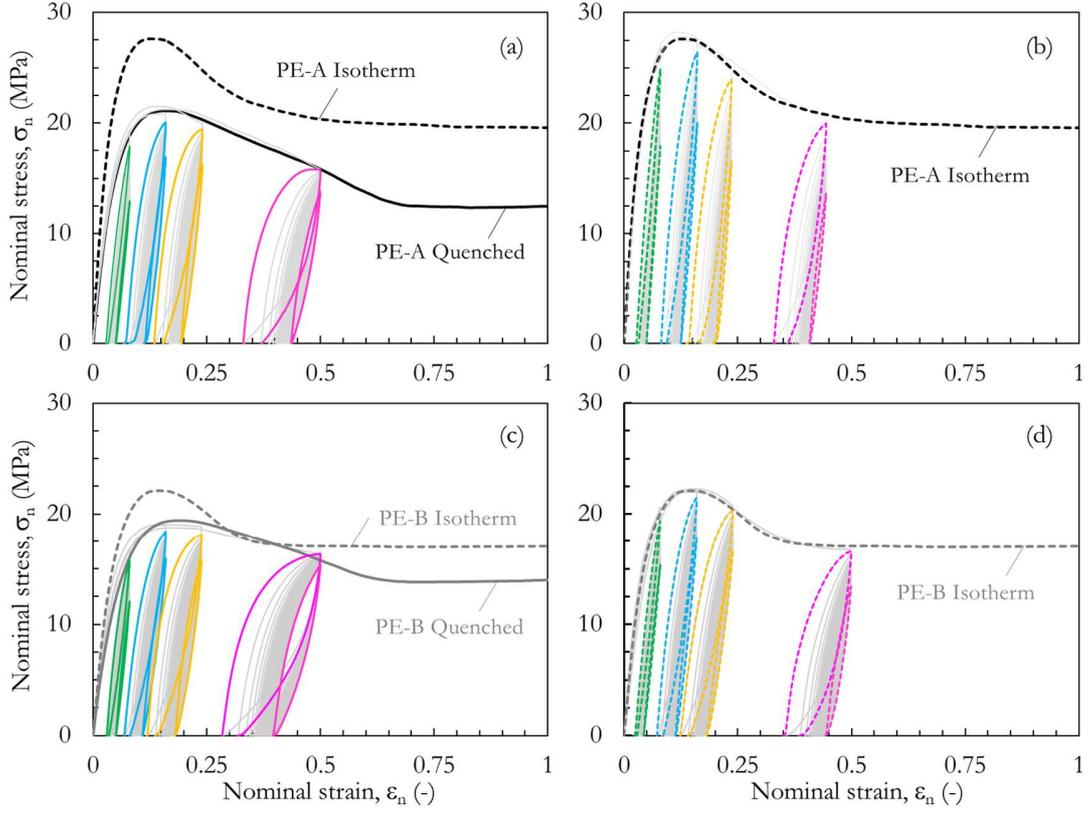
**Figure 1:** Nominal uniaxial and oligo-cyclic tensile stress-strain profiles.
