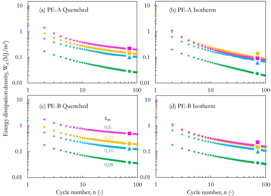
**Figure 7:** Density of energy dissipation  $W_d$  as a function of cycle number in PE samples with different applied oligo-cyclic strains  $\epsilon_{OC}$ : (a) PE-A Quenched; (b) PE-A Isothermal; (c) PE-B Quenched and (d) PE-B Isothermal
