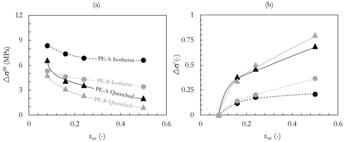
**Figure 4:** a) Total stress-softening magnitudes between 1<sup>st</sup> and 100<sup>th</sup> loading; b) Relative decrease of stress softening as a function of  $\epsilon_{OC}$  in different samples
