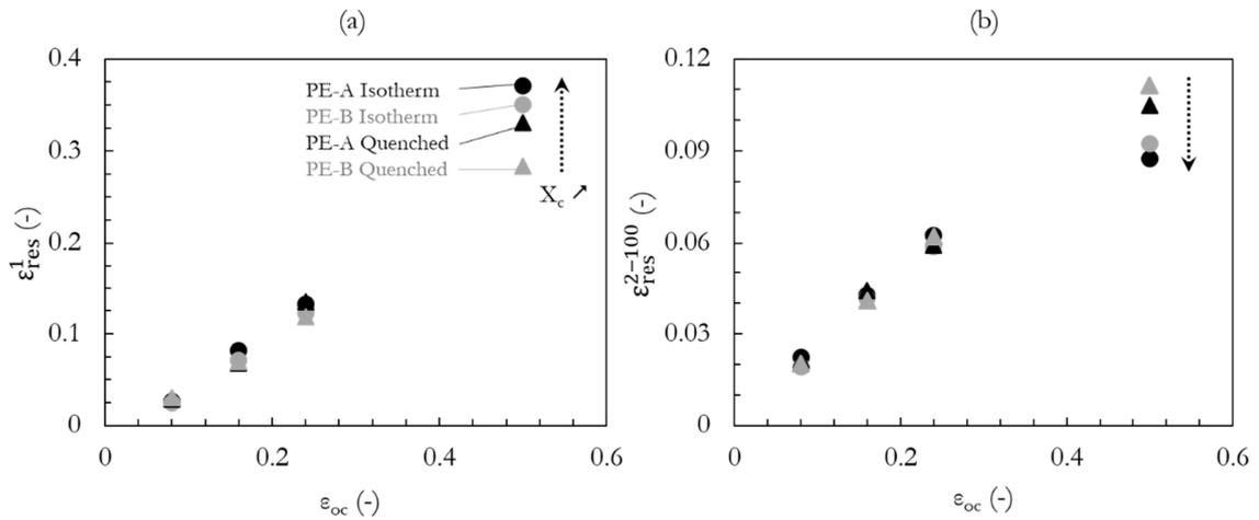
**Figure 6:** Change of the residual strains as a function of the prescribed maximum strain a) after the 1<sup>st</sup> cycle, b) from 2<sup>nd</sup> to 100<sup>th</sup> cycle
