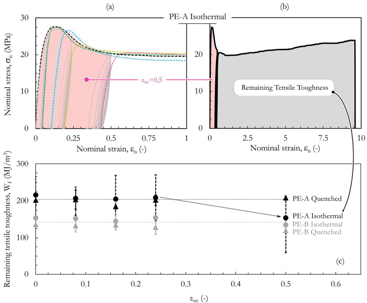
**Figure 12:** a) Mullins-like behavior of PE-A isothermal sample; b) Definition of remaining tensile toughness (ex. PE A isothermal sample, with  $\epsilon_{oc}=0.5$ ), c) Remaining tensile toughness in different samples as function  $\epsilon_{oc}$
