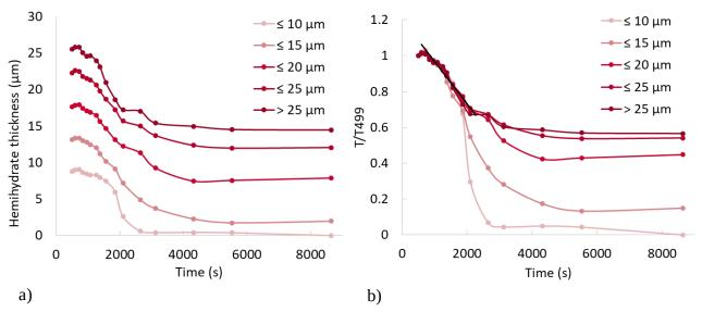
Figure 8: a) Hemihydrate thickness evolution during setting for different classes of initial particle thicknesses b) Normalized thickness evolution of hemihydrate particles. Measurements based on an average of 22 particles per size class.
