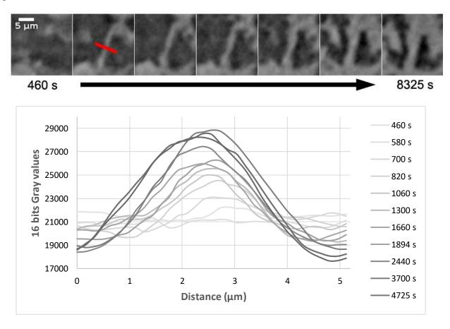
Figure 10: Top: Evolution versus time of the same 2D reconstructed slice showing the growth of a gypsum crystal, voxel size 0.163 µm. Bottom: gray level profiles across the forming gypsum crystal for different times. A small offset in distance can be observed for the two last curves at 6561 s and 8325 s as the stabilization of the images with time could not be performed perfectly.
