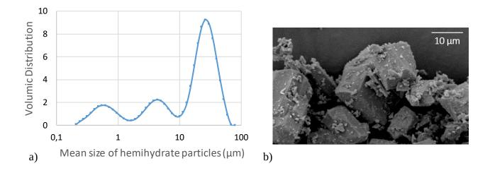
Figure 1: a) Particle size distribution in volume of the hemihydrate powder (n = 4). The plot represents the mean value of four measurements performed on different batches. b) SEM micrograph of the hemihydrate powder.
