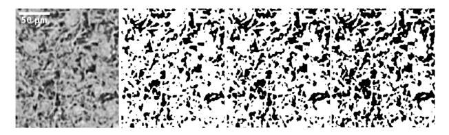
Figure 5: Section of a volume at 0.65 µm per voxel of entangled gypsum crystals. Same image before (left) and after binarization with different thresholds, i.e. a 16-bit gray value of 25700, 28270, and 30583 respectively (see Table 1)
