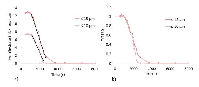
Figure 9: a) Hemihydrate thickness evolution during setting for two classes of smallest initial particle sizes b) Normalized thickness evolution versus time.
