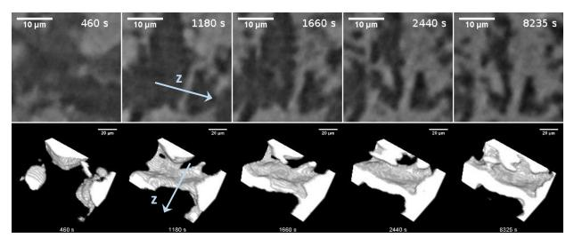
Figure 4: Illustration of the growth of a gypsum crystal. Evolution versus time of one same reconstructed 2D slice extracted from the 3D volumes acquired during the in situ tomography experiments with a voxel size of 0.163 µm, between 460 and 8325 s (top line) and associated 3D visualization (bottom line).
