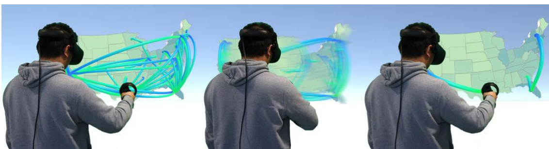
Figure 9. Embodied interaction for filtering by shaking the map. Left: before shaking, the map shows all flow symbols. Center: Shaking removes flows with small values. Right: After shaking, the map only shows flows with large values.
