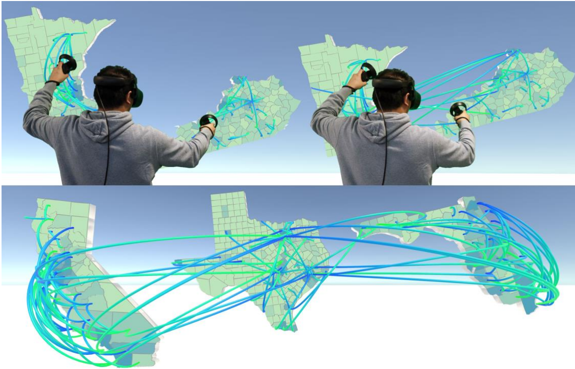
Figure 7. Embodied interaction for creating flow lines between two maps. Top left: maps are moved together. Top right: linking flow lines appear when the two maps are close enough. Bottom: An example of chained flow maps, where the user linked three maps together in a custom arrangement.
