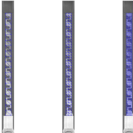
**Figure 5:** Three meshes used for the DIC analyses at the macroscale of the speckled surface
