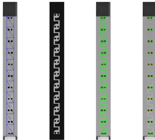
Figure 18: Backtracked meshes for microscale DIC of the dotted surface. The image of the reference configuration (leftmost) is registered with that of the nominal configuration (left) using the auxiliary mesh shown in blue. The backtracked mesh is laid over the reference image (right). The grain centers (red crosses) are also depicted. Similarly, the 4-element zones about each dot are also backtracked (rightmost)
