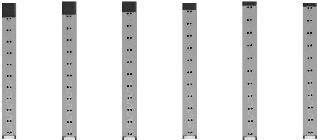
Figure 15: Cropped gray level images of the extensional test with dotted grains
