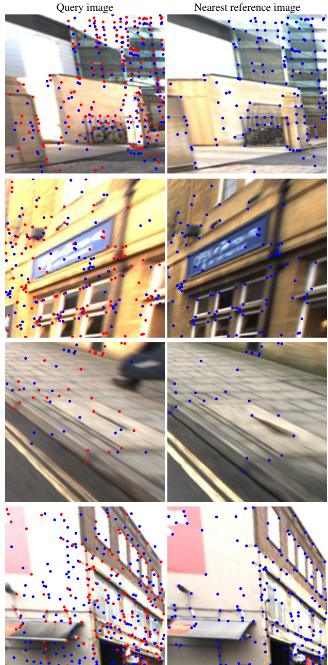
Figure 9. Inaccurate RobotCar ground truth poses. We plot the projection of 3D SfM points in the query images according to the ground truth (in blue) and hloc (in red) poses. We project the same points in the reference images using the reference poses (in blue). Query points using hloc are better aligned to the reference points, indicating that the ground truth query poses are inaccurate.
