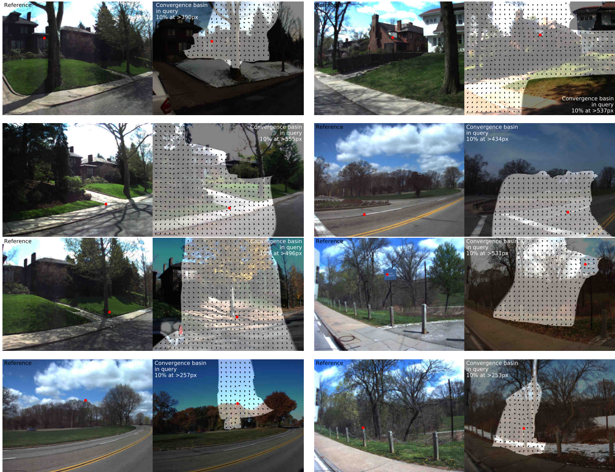
Figure 14. Convergence basin. We show the convergence basins of individual selected points given cross-season query and reference images from the CMU dataset. The last row shows smaller basins due to repeated patterns like poles or tree silhouettes.
