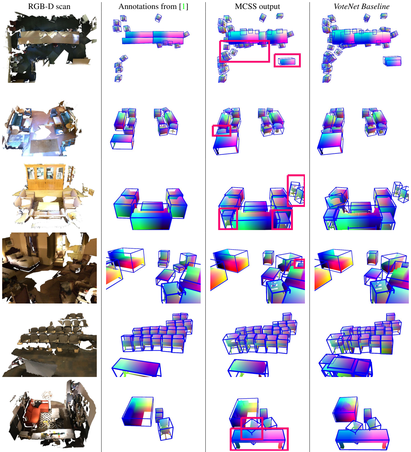
Figure 8: RGB-D scans from ScanNet [5], existing manual annotations, output of our MCSS approach, and output of VoteNet for object 3D pose and model retrieval. Note we retrieve objects (shown in red boxes) that are not in the manual annotations, and that VoteNet tends to miss objects or recover an incorrect pose or model when objects are close to each other.
