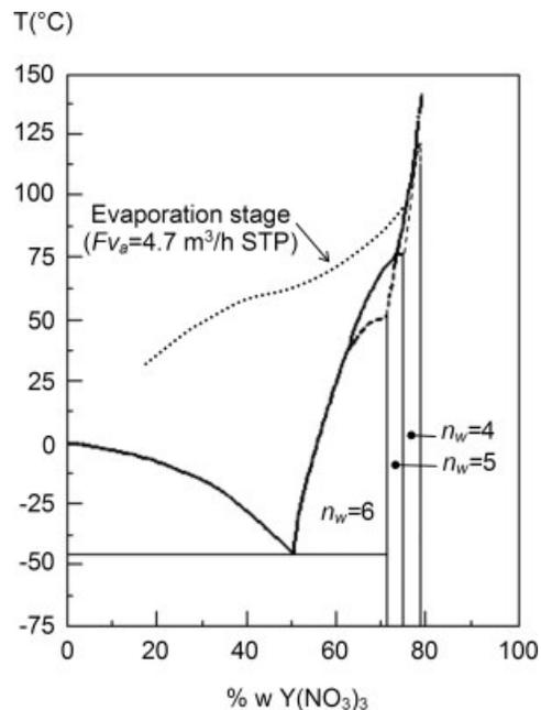
Figure 4. Binary diagram for the  $\text{H}_2\text{O}-\text{Y}(\text{NO}_3)_3$  system<sup>26</sup>—domains of solid  $\text{Y}(\text{NO}_3)_3 \cdot n_w \text{H}_2\text{O}$  indicated by the values of  $n_w$ .
