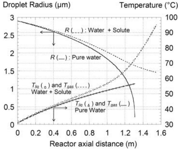
**Figure 1. Variation of the droplet radius, gas and liquid temperatures along the reactor axis for pure water and (water +  $Y^{3+}/NO_3^-$ )— $Fv_a = 4.7 \text{ m}^3/\text{h}$  STP,  $Fv_w = 0.32 \text{ l/h}$  STP,  $R_0 = 2.9 \text{ } \mu\text{m}$ .**
