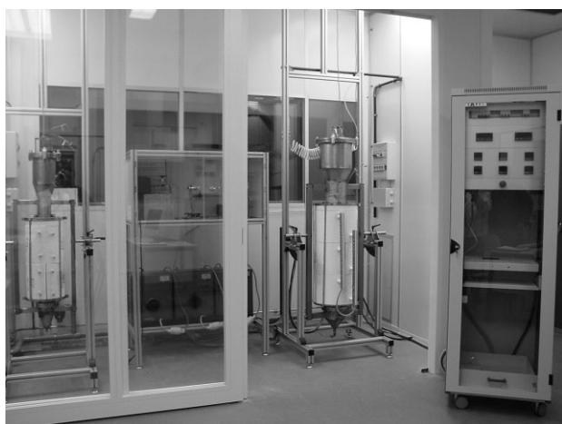
Fig. 11. Photographs of the 5.3 cm i.d. and the 16 cm i.d. FB-CVD reactors.
