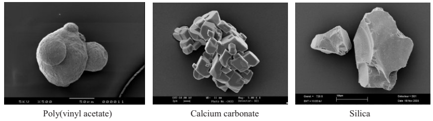
Fig. 1: SEM photos of the products.
