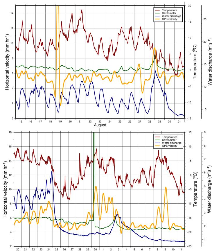
The significant speed-up event (~9 mm h<sup>-1</sup>) happened in the day boundary between August 28 and 29, presumably attributed to the excessive precipitation given water discharge increase and air temperature drop. The cavitometer also registered this speed-up event with slightly less magnitude ~8.5 mm h<sup>-1</sup>. The compressive strain rates increased on August 28 reflecting the speed-up event.
