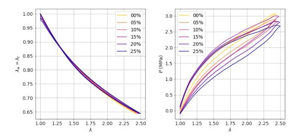
Figure 7: Lateral stretch ratio (left) and nominal stress (right) vs. stretch ratio for all materials.
