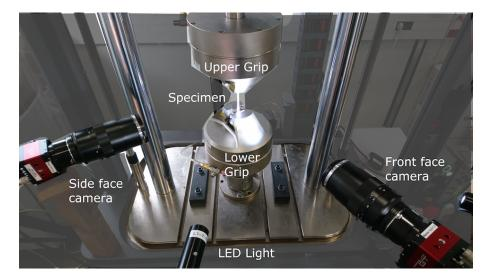
Figure 2: Experimental set-up with camera positioning.
