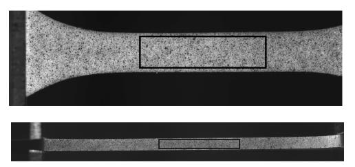
Figure 3: Virtual strain gauges on undeformed samples. Top: front face. Bottom: side face.
