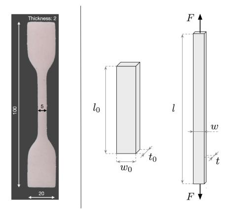
Figure 1: Sample. Left: dimensions (mm). Right: notations.
