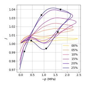
Figure 9: Volumetric response of the six materials.
