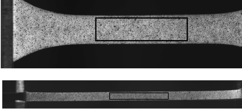
Figure 3: Virtual strain gauges on undeformed samples. Top: front face. Bottom: side face.
