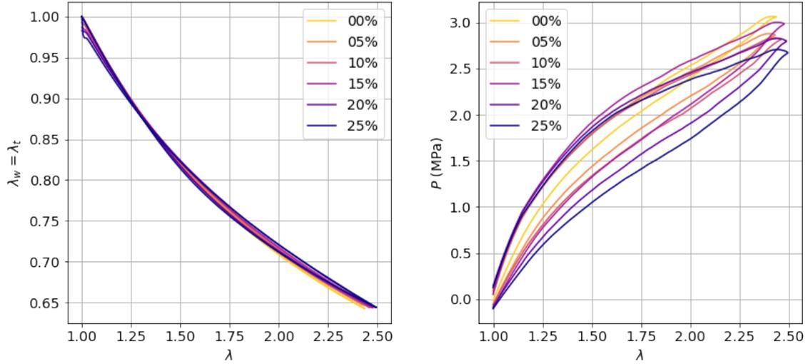
Figure 7: Lateral stretch ratio (left) and nominal stress (right) vs. stretch ratio for all materials.
