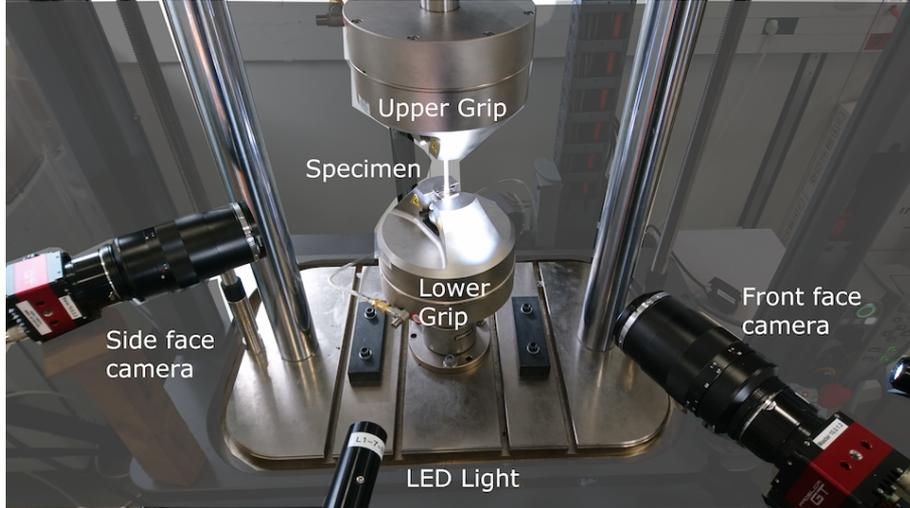
Figure 2: Experimental set-up with camera positioning.
