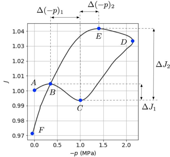
Figure 10: Description of the volumetric response. Definition of the extrema and the jumps, example of the 25% filled material.
