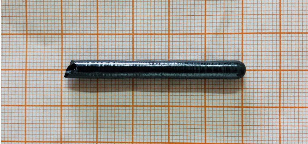
Fig. S1: Single Crystal. Picture of YFeO 3 single crystal grown by optical float-zone method.
