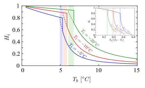
Fig. 7: Theoretical prediction of the bistability phenomena for RB case:  $H_i$  as a function of  $T_b$  for three different cold plate temperatures,  $T_t = -5^{\circ}\text{C}$  (blue curves),  $T_t = -10^{\circ}\text{C}$  (red curves), and  $T_t = -20^{\circ}\text{C}$  (green curves). The blue, red, and green shaded areas correspond to the bisability regime for the three values of  $T_t$  respectively. The inset is  $H_i$  as a function of the normalized temperature  $T_b/(T_b - T_t)$ .
