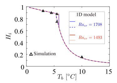
Fig. 6: Theoretical prediction of the bistability phenomena for RB case:  $H_i$  as a function of  $T_b$  The red and blue curves correspond to the model prediction using  $Ra_{cr}=1493$  and  $Ra_{cr}=1708$  respectively, for the condition of  $T_t=-10^{\circ}$ . The symbols are results from the simulation.
