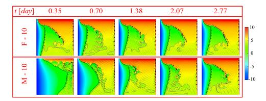
Fig. 11: The evolution of the instantaneous temperature field of the freezing process (top row) and melting process (bottom row), with the bottom plate temperature  $T_b = 10^{\circ}$  C. The black and blue thick lines denote the ice-water interface with temperature  $0^{\circ}$  C and the density peak temperature (i.e.,  $4^{\circ}$ C) isotherm, respectively. The arrows denotes the velocity vectors.
