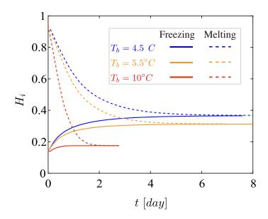
Fig. 8: Evolution of the ice thickness,  $H_i$ , of the freezing process (thick line) and the melting process (dashed line) for the three thermal driving conditions (i.e.,  $4.5^{\circ}$ C,  $5.5^{\circ}$ C, and  $10^{\circ}$ C, respectively)
