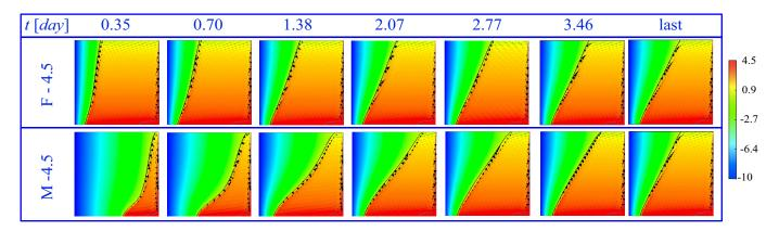
Fig. 9: The evolution of the instantaneous temperature field of the freezing process (top row) and melting process (bottom row), with the bottom plate temperature  $T_b = 4.5^{\circ}$ C. The black and blue thick lines denote the ice-water interface with temperature  $0^{\circ}$ C and the density peak temperature (i.e.,  $4^{\circ}$ C) isotherm, respectively. The arrows denotes the velocity vectors.
