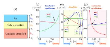
Fig. 2: Mechanism of bistability: (a) Sketch of the onedimensional model: three plane layers are connected in series. Note that if  $T_b < T_c$  the unstably stratified layer is absent; The computed heat-fluxes across the cell as a function of the ice thickness,  $h_i$ , in the purely conductive regime (b), the bistable regime (c) and the convective one (d).
