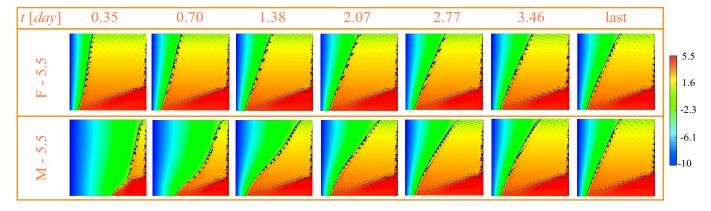
Fig. 10: The evolution of the instantaneous temperature field of the freezing process (top row) and melting process (bottom row), with the bottom plate temperature  $T_b = 5.5^{\circ}$ C. The black and blue thick lines denote the ice-water interface with temperature  $0^{\circ}$ C and the density peak temperature (i.e.,  $4^{\circ}$ C) isotherm, respectively. The arrows denotes the velocity vectors.
