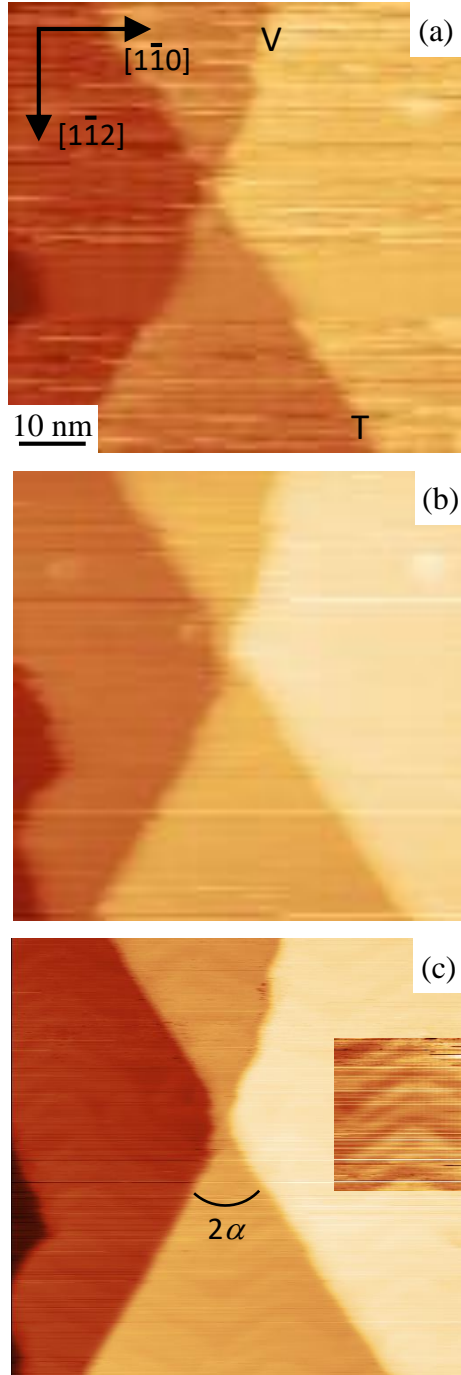
Figure 3: Characteristic kinetic evolution of the Au(111) surface for 2\alpha = 60^\circ during the anticrossing phenomenon (UHV-STM investigations at T = 297 K) at (a) t = 40 s, (b) 370 s and (c) 760 s after the emergence of the slip trace. In the inset, the contrast is enhanced to highlight the well-known herringbone pattern characteristic of the Au(111) atomic reconstruction. V and T correspond to a vicinal step and a slip trace, respectively.
