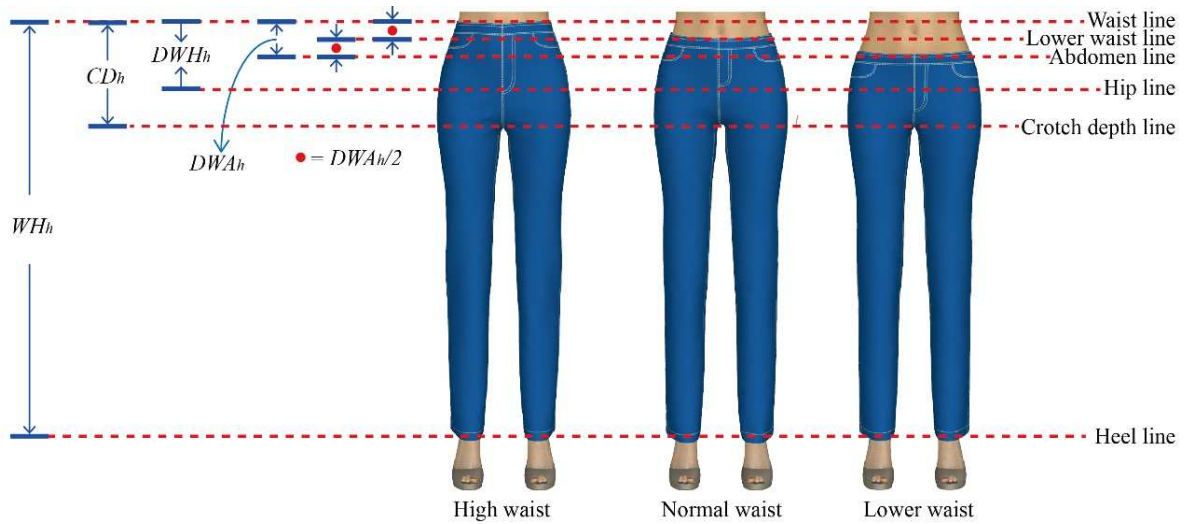
2 Fig. 4. Jean waist design. ( WH_h is human body waist height; CD_h is human body crotch depth; DWH_h is 3 human body drop of waist-to-hip; DWA_h is human body drop of waist-to-abdomen.)
