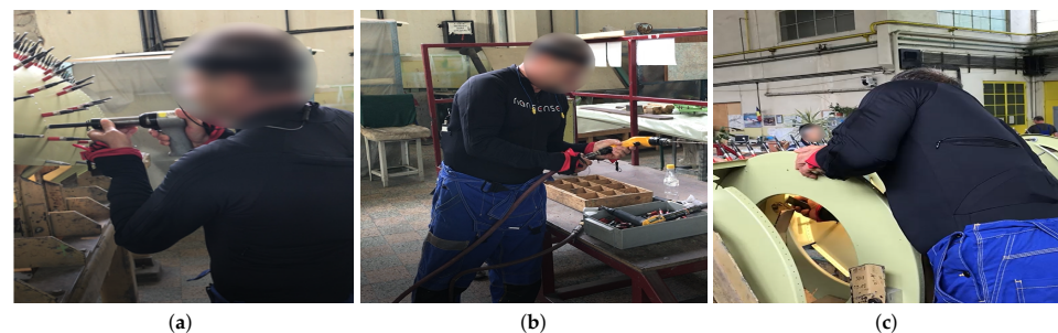
Figure 3. Gesture vocabulary with gestures for airplane assembly ( G_2 ). (a) G_{2,1} : Rivet with the pneumatic hammer; (b) G_{2,2} : Prepare the pneumatic hammer and grab rivets; (c) G_{2,3} : Place the bucking bar to counteract the incoming rivet.
