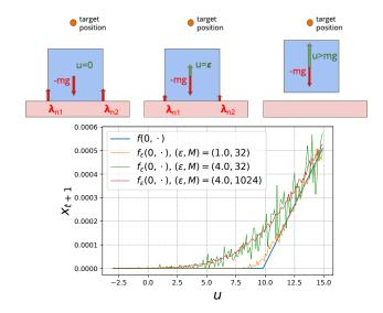
Fig. 2: **Top:** A slight vertical force is not able to break the unilateral contact, leaving cube on the floor and, thus, the state unchanged. **Bottom:** The non-smoothness of physics induces null gradients  $\nabla_{\boldsymbol{u}} R$  which results in the failure of classical optimization techniques (III-A).
