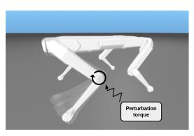
Fig. 1: Illustration of randomized smoothing effects on the front left leg of the Solo robot.
