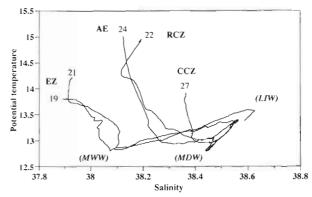
Fig. 4. Potential temperature (°C)/salinity diagrams for some selected stations of the 4 hydrological zones: EZ: external zone: Stns 21, Riviera and 19, Corsica; RCZ: Riviera coastal zone; AE: anticyclonic eddy; and CCZ: Corsica coastal zone. Position of type waters: MWW: Mediterranean Winter Water; LIW: Levantine Intermediate Water, and MDW: Mediterranean Deep Water
