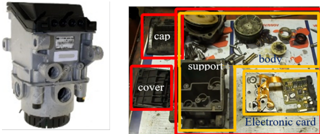
Fig. 4. EBS module and components of the returned module (Bentaha, et al 2020).
