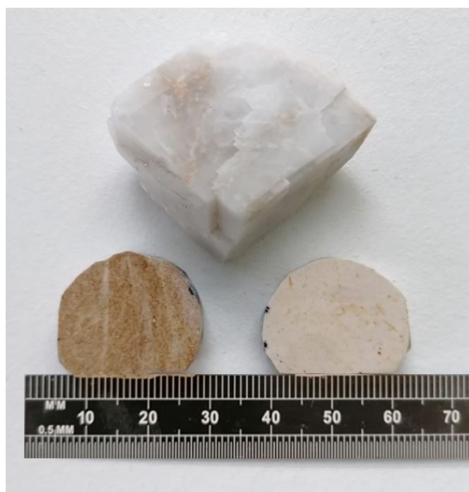
Figure 5. Cylindrical rock plugs of Ciply Chalk ( bottom left ) and Obourg Chalk ( bottom right ), and pure single calcite ( top ) used for surface characterization. The scale is given by the ruler in mm.
