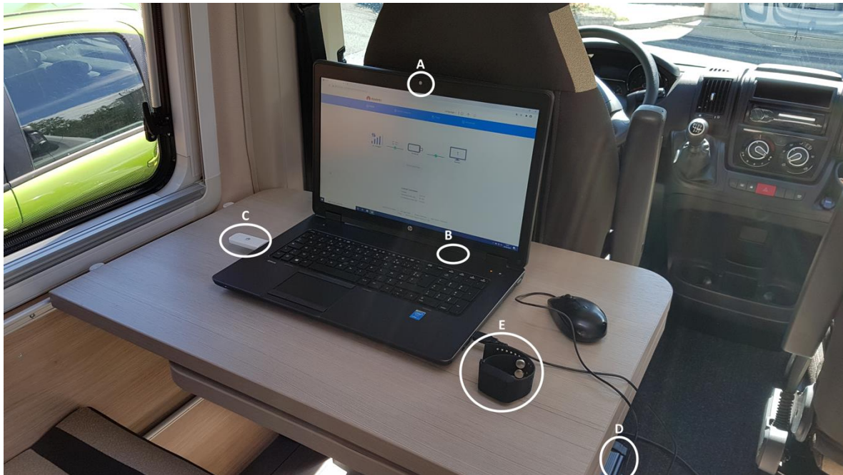
Figure 3. The laptop from the participants' side (A) integrated microphone and webcam. (B) integrated speakers. (C) 4G key for internet connection. (D) Converter battery attached to the van's electric plug to charge the laptop. (E) Empatica E4 wristband for stress measurement retrieval.
