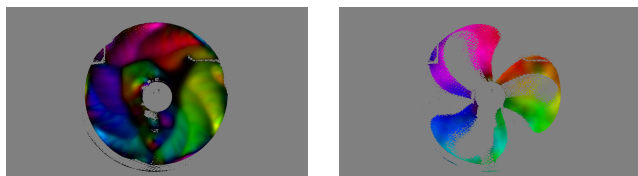
Fig. 8. Sample EBOF results for the “Fan” sequence of our high-speed dataset, with \Delta T = 15\text{ms} (left) and \Delta T = 5\text{ms} (right). Notice how the blades of the fan are merged together in the first case, while they appear clearly in the second one, leading to improved optical flow results.
