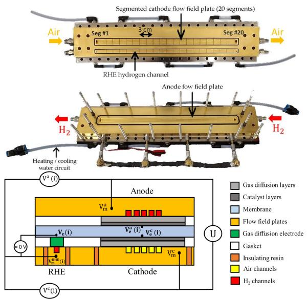
**Figure 1**. Pictures and operation principle of the linear segmented cell. Up: segmented cathode flowfield with the auxiliary hydrogen channel feeding the RHE used to measure the local potentials. Middle: anode flow-field plate. Bottom: cross-sectional view of the cell. The reference electrodes give access to the local electrolyte potential  $V^{e}(i)$  and thus to the anode and cathode potentials of each segment [<sup>22,35</sup>].
