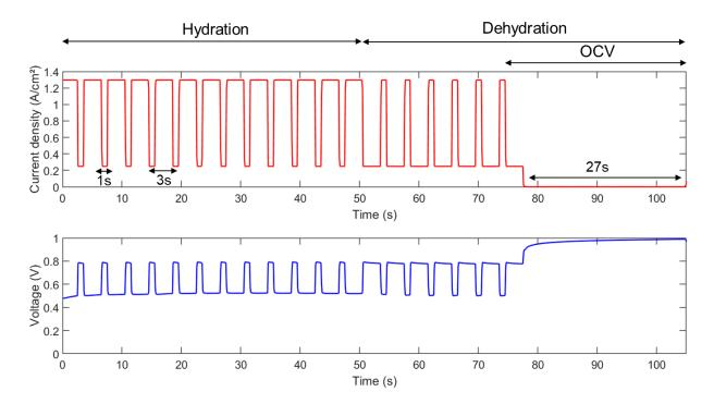
**Figure 3.** Current density and voltage profiles during the RH and load cycling AST. The hydration stage consists of alternating 1 s at low current ( $0.25 \text{ A/cm}^2$ ) and 3 s at high current ( $1.3 \text{ A/cm}^2$ ) sequences and lasts 52 s. The dehydration stage consists of alternated sequences of 3 s at low current and 1 s at high current, followed by 27 s at OCV (total duration = 105 s) [<sup>22</sup>].
