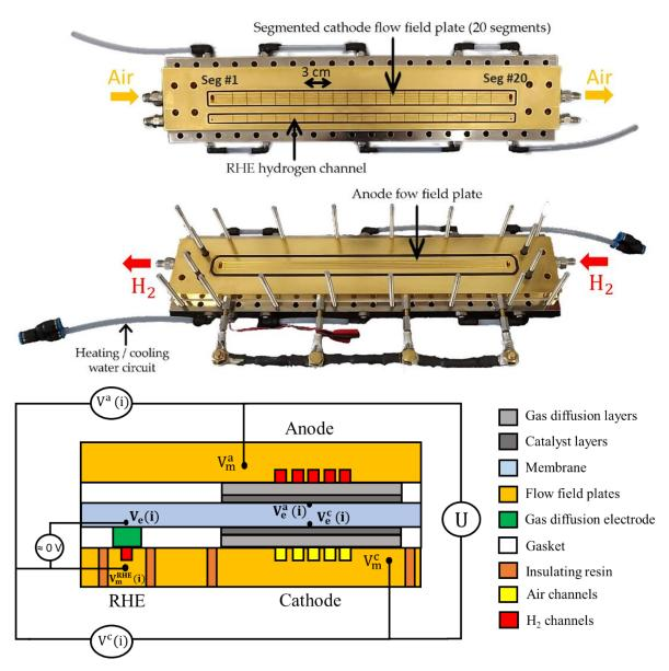
**Figure 1**. Pictures and operation principle of the linear segmented cell. Up: segmented cathode flow-field with the auxiliary hydrogen channel feeding the RHE used to measure the local potentials. Middle: anode flow-field plate. Bottom: cross-sectional view of the cell. The reference electrodes give access to the local electrolyte potential  $V^{e}(i)$  and thus to the anode and cathode potentials of each segment [<sup>22,35</sup>].
