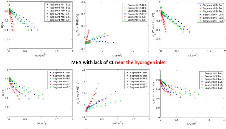
MEA with lack of CL near the hydrogen outlet
