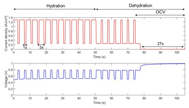
**Figure 3.** Current density and voltage profiles during the RH and load cycling AST. The hydration stage consists of alternating 1 s at low current (0.25 A/cm<sup>2</sup>) and 3 s at high current (1.3 A/cm<sup>2</sup>) sequences and lasts 52 s. The dehydration stage consists of alternated sequences of 3 s at low current and 1 s at high current, followed by 27 s at OCV (total duration = 105 s) [<sup>22</sup>].
