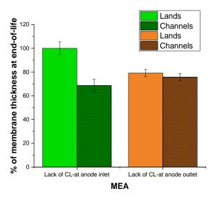
**Figure 7**. EoT membrane thickness compared to BoL (100%), below the channels and below the lands, in the segments with a lack of anode CL (*i.e.* #3 in the case of the MEA with a lack of anode CL near the hydrogen outlet, and #18 in the case of the MEA with a lack of anode CL near the hydrogen inlet). Data plotted on the graphs correspond to the average values of five measurements, with standard deviation.
