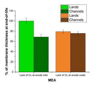
**Figure 7**. EoT membrane thickness compared to BoL (100%), below the channels and below the lands, in the segments with a lack of anode catalyst layer (*i.e.* #3 in the case of the MEA with a lack of anode CL near the hydrogen outlet, and #18 in the case of the MEA with a lack of anode CL near the hydrogen inlet). Data plotted on the graphs correspond to the average values of five measurements, with standard deviation.
