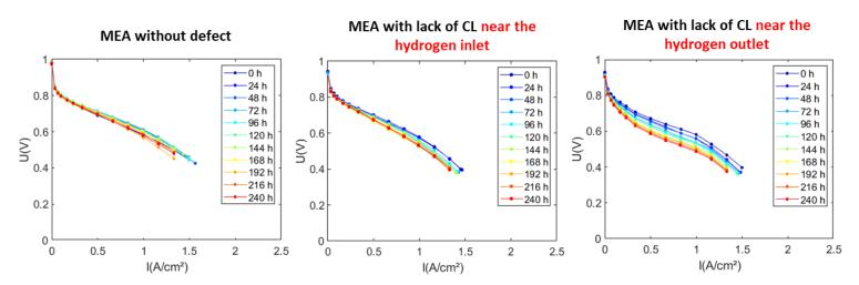
**Figure S1**. Polarization curves measured every 24 hours during the AST, with the MEA without defect (right), with the MEA with a lack of anode CL near the hydrogen inlet (center) and near the hydrogen outlet (right).
