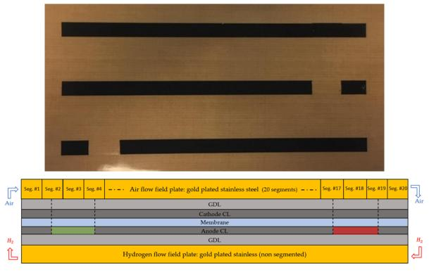
**Figure 2**. Up: anode -before transfer on the membrane- with -or without- a lack of CL at one end. Below: longitudinal sectional view of the segmented cell. The location of the defect is situated either at the anode inlet (in green) or outlet (in red).
