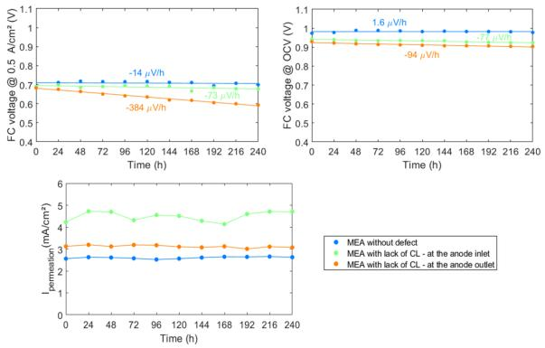
**Figure 4.** Variation of the FC voltage at 0.5 A/cm<sup>2</sup> (top, left), of the OCV (top, right) and of the hydrogen permeation current (bottom) during AST performed with a reference MEA (without defect), a MEA with a lack of anode CL close to the hydrogen inlet, and a MEA with a lack of anode CL close to the hydrogen outlet. All data were measured during the characterization stage performed every 24 h. The voltage degradation rates were estimated using a linear interpolation of the dots.
