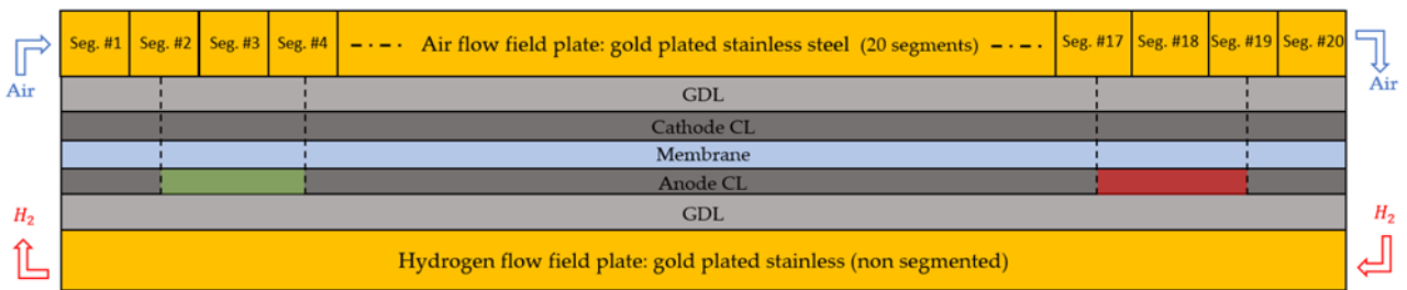
Figure 2. Up: anode -before transfer on the membrane- with -or without- a lack of CL at one end. Below: longitudinal sectional view of the segmented cell. The location of the defect is situated either at the anode inlet (in green) or outlet (in red).
