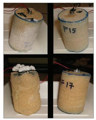
**5.** - Samples after weathering cycles with  $CaSO_4$  (up) and  $Na_2SO_4$  (bottom) under low relative humidity conditions (left) and high relative humidity (right).
