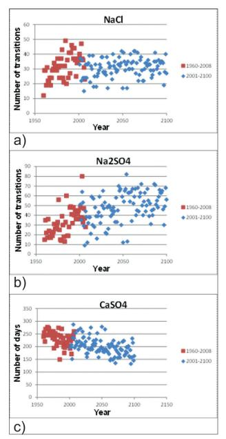
**7.** - Evolution of "salt weathering" with time. (a) Number of NaCl precipitation by decrease of the relative humidity. (b) Number of thenardite mirabilite transitions. (c) Number of days with relative humidity higher than 80% (for CaSO<sub>4</sub> crystallization).
