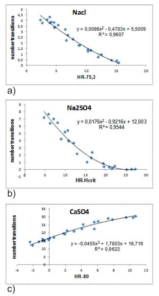
**9.** - Average number of transitions per month calculated from observed data at Rouen and Caen versus the difference between relative humidity and equilibrium relative humidity for each salt system.
