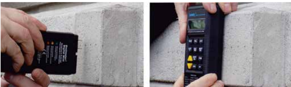
Figure 6. Left: Pin moisture meter (Protimeter), right: pinless moisture meter (Tramex).
