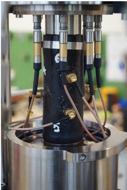
Fig. 4 Rock sample jacketed with a neoprene sleeve with PZT transducers in place
