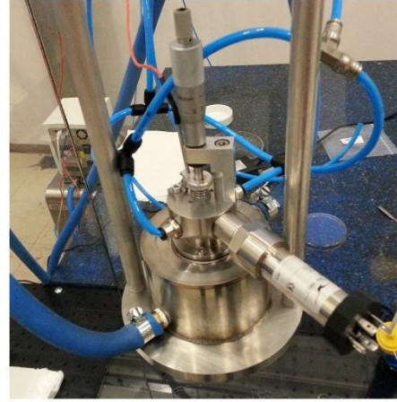
Figure 3: Drop on demand device. The liquid metal is contained in the red part (online version) while gas is supplied and exits through the green part (online version). The yellow (online version) stopper rod is slightly open preventing dripping when a gas over-pressure is not provided.
