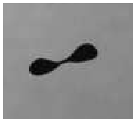
Figure 7: We = 21 breakup of a droplet into two equals parts. Heating of the surrounding fluid leads to a slight blur around the droplet.
