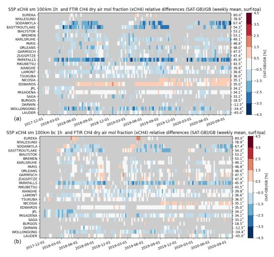
Figure 3. Mosaic plots showing relative biases between co-located S5P (standard XCH<sub>4</sub> product - a; bias-corrected XCH<sub>4</sub> product - b) and TCCON XCH<sub>4</sub> data with a priori alignment at 25 TCCON stations within the period between November 2017 and September 2020. Spatial co-location with radius of 100 km and time of  $\pm 1$  h around the satellite overpass was used. The time resolution of the data shown here is weekly. The stations are sorted with decreasing latitude.
