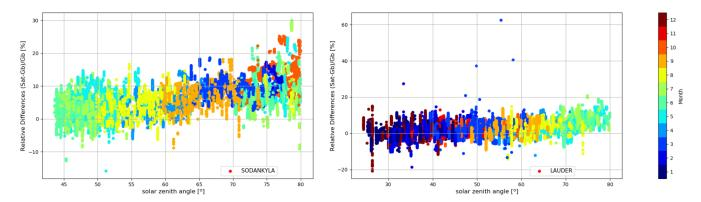
**Figure 35.** Relative biases between co-located S5P XCO and TCCON unscaled XCO data with a priori aligned are plotted as a function of the S5P measurement solar zenith angles retrieved at a few TCCON stations within the period between November 2017 and September 2020. Spatial co-location with radius of 50 km and time of  $\pm 1$  h around the satellite overpass was used. The colours represent the different months from January (1) until December (12) of a year.
