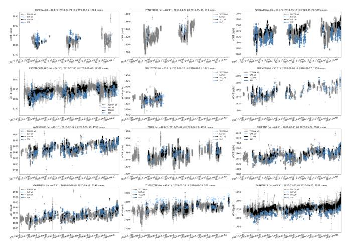
Figure 4. XCH<sub>4</sub> time series for all TCCON data (grey), S5P bias-corrected data (light blue), S5P data co-located with TCCON data (blue) and co-located TCCON data with a priori alignment (black) at each site ordered with decreasing latitude. Spatial co-location with radius of  $100 \, \text{km}$  and time of  $\pm 1 \, \text{h}$  around the satellite overpass was used.
