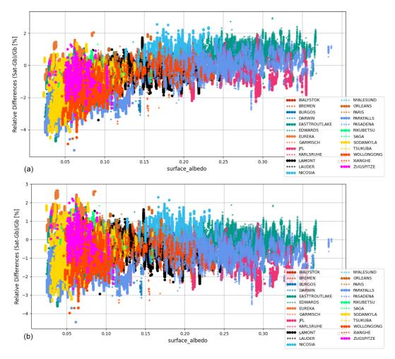
Figure 2. Relative biases between co-located S5P (standard XCH<sub>4</sub> product –  $\mathbf{a}$ ; bias-corrected XCH<sub>4</sub> product –  $\mathbf{b}$ ) and TCCON XCH<sub>4</sub> data with a priori alignment are plotted as a function of the surface albedo retrieved by S5P at 25 TCCON stations within the period between November 2017 and September 2020. Spatial co-location with radius of 100 km and time of  $\pm 1$  h around the satellite overpass were used.
