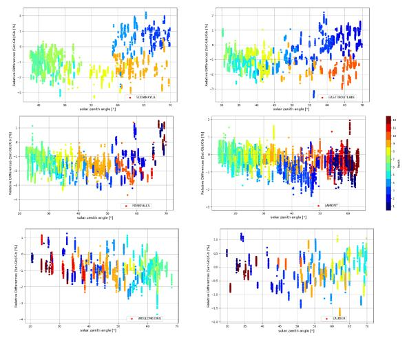
Figure 17. Relative biases between co-located S5P bias-corrected XCH<sub>4</sub> and TCCON XCH<sub>4</sub> data with a priori alignment are plotted as a function of the S5P measurement solar zenith angles retrieved at a few TCCON stations within the period between November 2017 and September 2020. Spatial co-location with radius of 100 km and time of  $\pm 1$  h around the satellite overpass was used. The colours represent the different months from January (1) until December (12) of a year.
