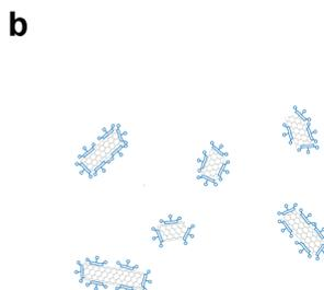
Figure 2. Possible effect of oxidation debris on the bundling behavior of (a) long CNTs, suggesting the formation of bundles, and (b) short CNTs, suggesting the formation of micelle-like structures.
